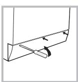
1. using a screwdriver, remove the cover panel on the lower front part of the washing machine (see figure);
